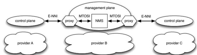
Fig. 1. Proxy between control plane and management plane
