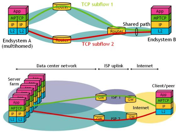
Figure 1: Multipath transport in general and in datacenter networks
