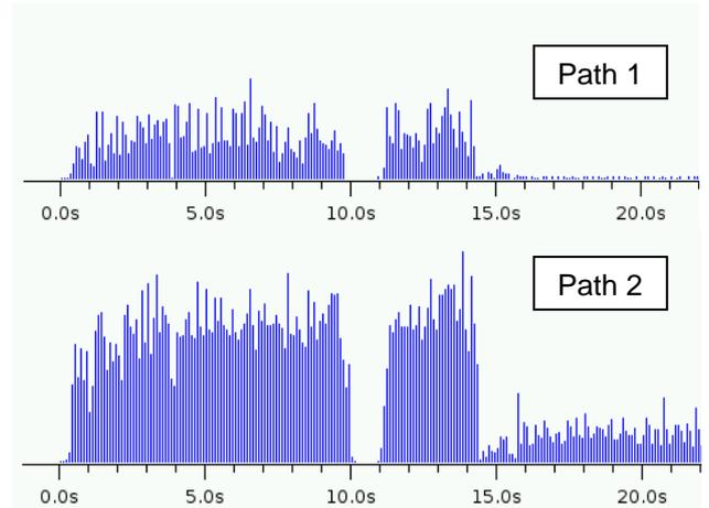
Figure 2: Bandwidth sharing measurement of user-space MPTCP
